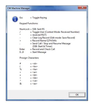
OK – that was a mouthful to digest. So let's do something simple first. Don't attach your keyer to a transmitter yet :-). To hear what the keyer is sending you have to enable the **Tone On** function, either using the keyer menus or the Configuration screen of the CW Machine Manager. Let's have the keyer send some text that you type in (make sure that the **Transmit Buffer** box has the yellow background – if not, left-click on it with your mouse).
